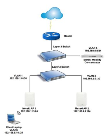
The diagram below shows the traffic flow for a particular flow within a campus environment using the Layer 3 roaming with concentrator.
