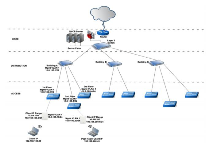
With layer 3 roaming, a client device must have a consistent IP address and subnet scope as it roams across multiple APs on different VLANs/subnets. Meraki's auto-tunnelling technology achieves this by creating a persistent tunnel between the L3 enabled APs and depending on the architecture a Mobility Concentrator. The two Layer 3 roaming architectures are discussed in detail below.
